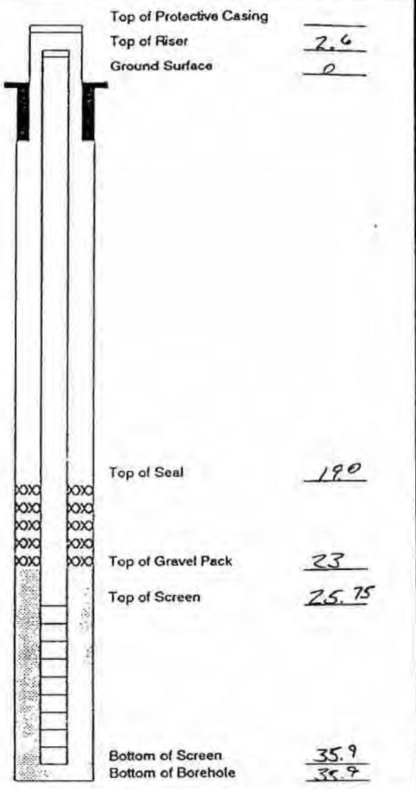
Comments: SAND Bridged in Auger hole to 22.4' below water. USED 9.5 BAG SAND (50#), 2.50# BAG'S Hole Plug, 3 BAG'S PORTLAND, 1/4 BAG Bentonite Powder. WL after install in 32 # BGS
