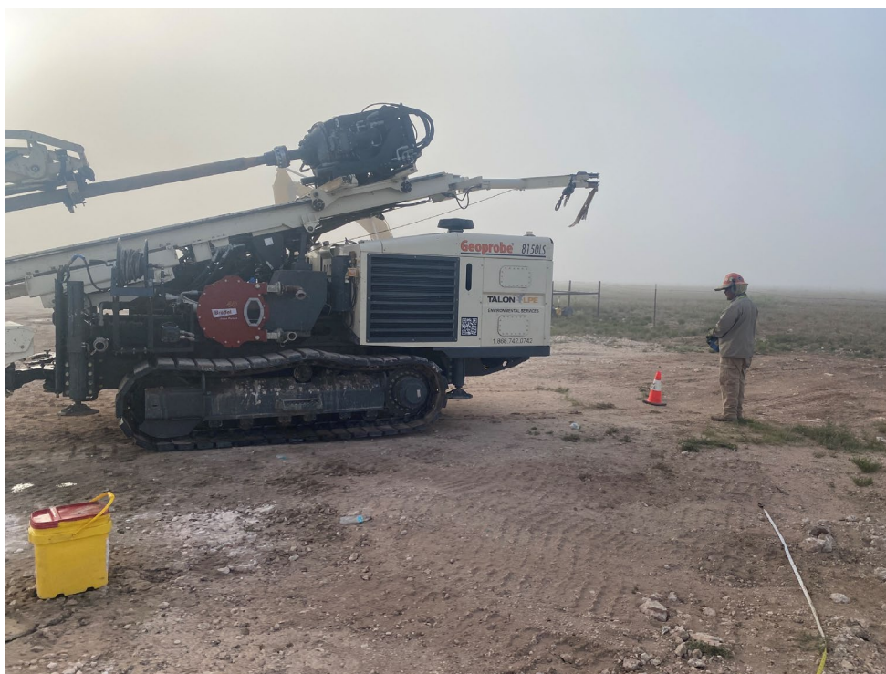
Photograph 1: Positioning track mounted sonic core rig over marked borehole location
