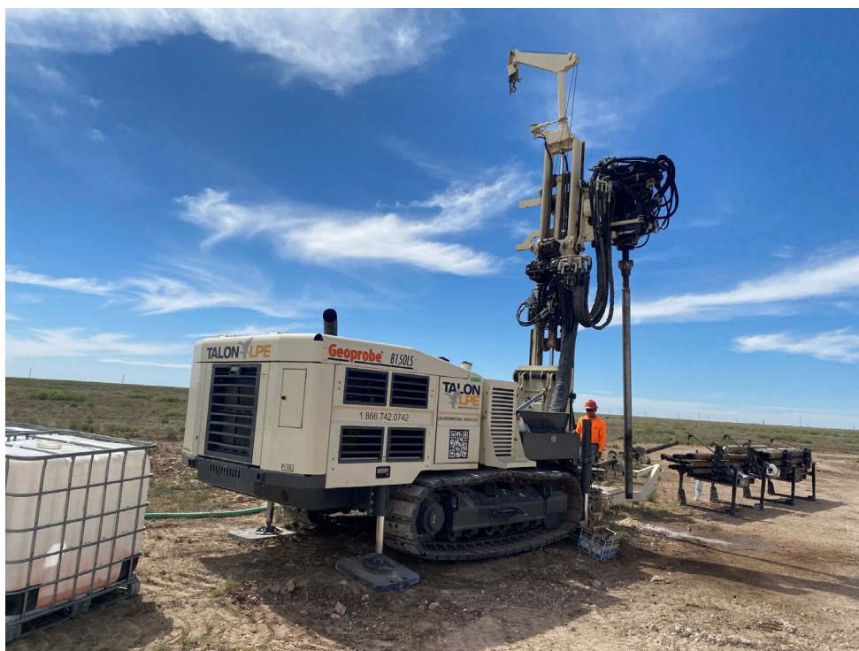
Photograph 2: Talon LPE – typical Geoprobe 8150LS sonic drill rig setup
