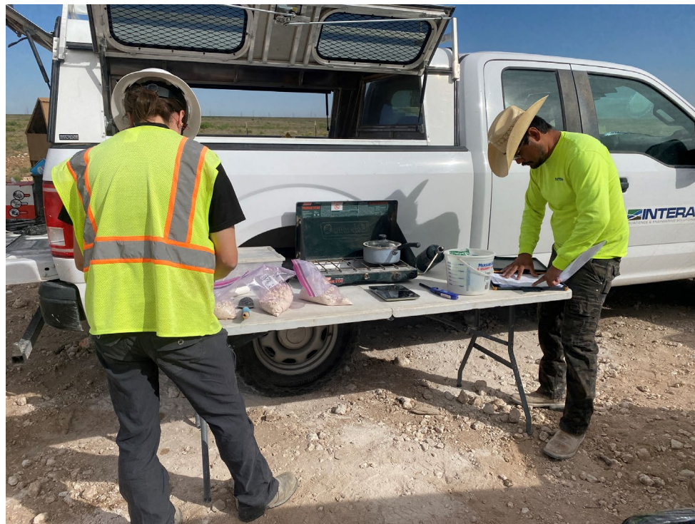
Photograph 6: INTERA geologists logging and field screening drilling samples for hydrocarbons and chlorides
