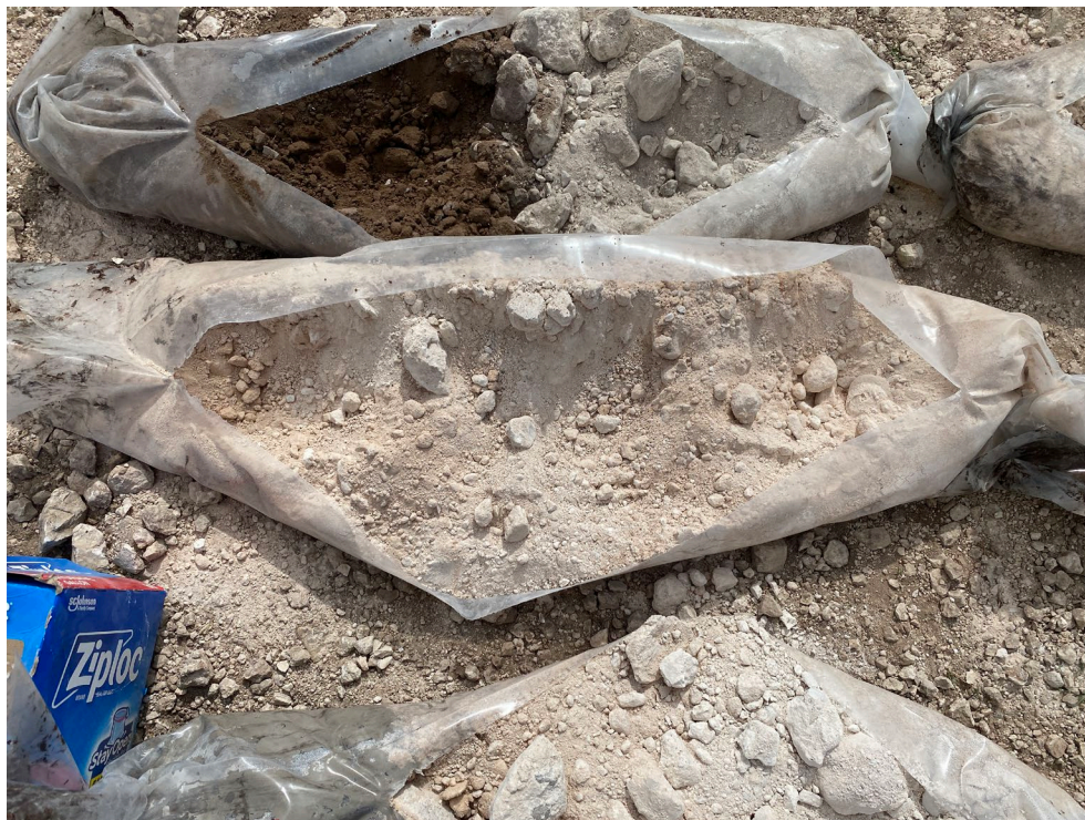
Photograph 5: Sonic core samples of dark sandy top soil and lighter colored caliche material
