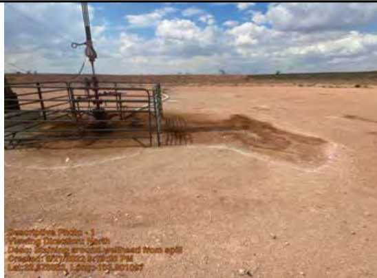
Staining around wellhead from spill
