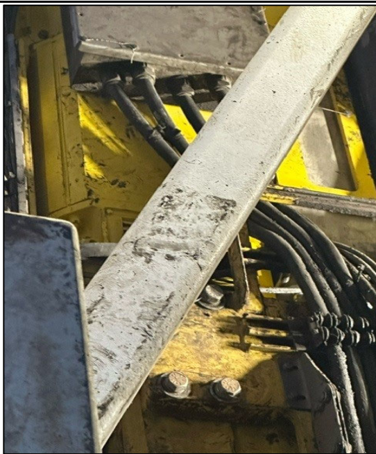
Photograph: 4 Date: 7/18/2024 Description: Damage to wiring that caused the fire. No fluids were released, but the Incident was reported because of the occurrence of a fire.
