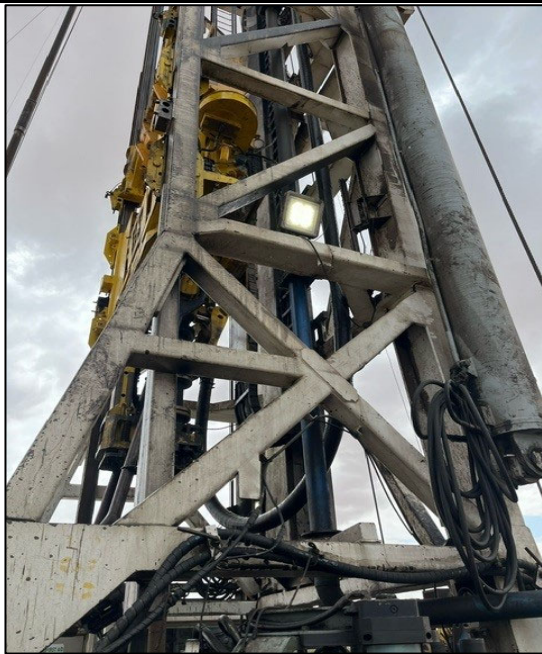
Photograph: 1 Date: 7/18/2024 Description: View of top drive showing the location of equipment where the fire occurred.
