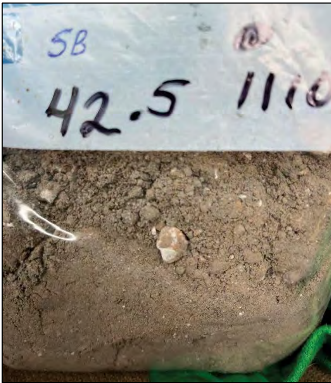
42.5 ft-sample : Silt with dolomite
