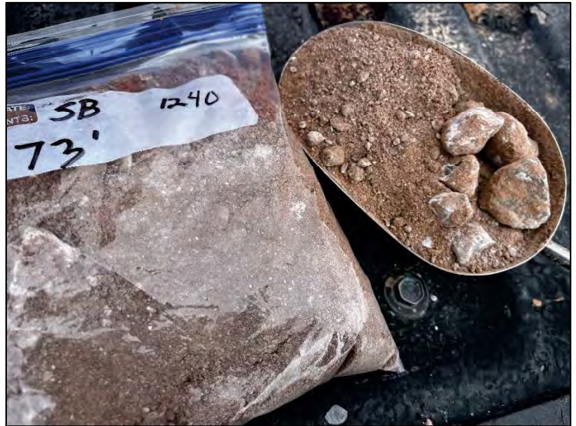
73-ft sample : auger (left), silt with limestone or dolomite (above)
