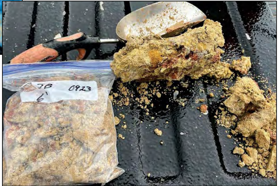
6-ft sample : appearance of red clay at bottom of auger
