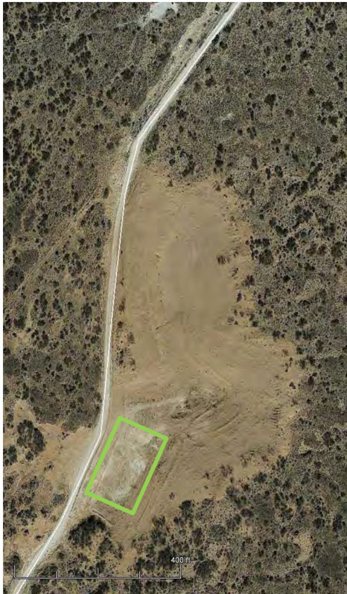
Figure C-1 – Location of phyto-remediation cell (green outline) in restored caliche pit. This area is exposed caliche and would benefit from the addition of sand/soil and seeding as proposed. Phytoremediation, not Micro-Blaze treatment is proposed for this cell.
