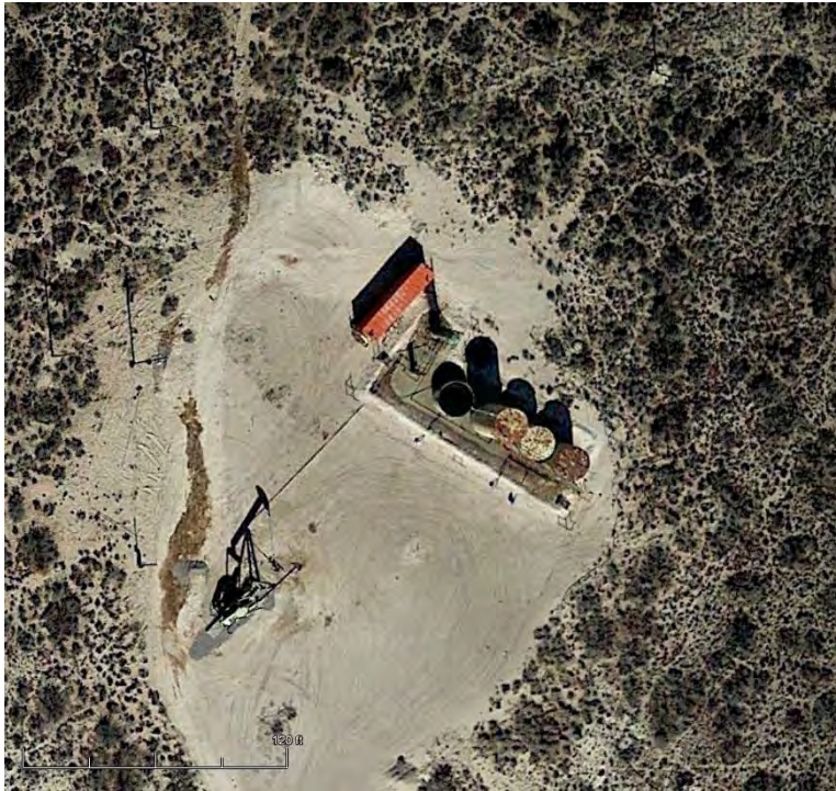
Figure 2 – This recent Google Earth image shows crude staining on the location as well as some staining off location on the abandoned dirt road on the northwest side of the image.
