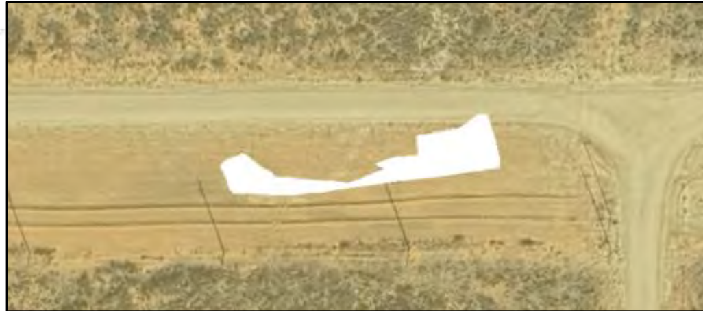
Figure 2. Aerial image of spill area. White polygon represents the spill area, overlapping primarily with a pipeline ROW and slightly with an adjacent graded road. Remediation activities are planned to be confined to these disturbed areas.
