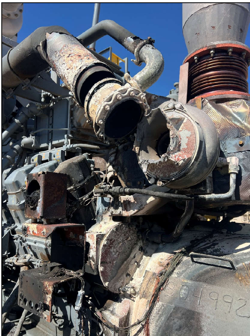
Photo of loose elbow on the turbo for unit 804992
