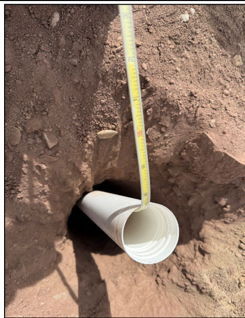
Photograph: 4 Date: 3/28/2025 Description: BH01 DTW ~54.75' BGS View: N/A
