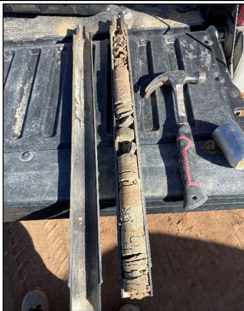
Photograph: 3 Date: 3/26/2025 Description: Boring BH05@5' split spoon interval View: North
