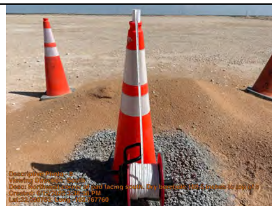
Northwest corner of pad facing south. Dry borehole 109.5 inches to top of casing.
