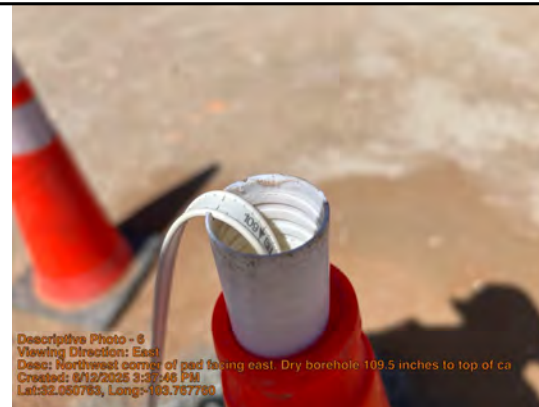
Northwest corner of pad facing northeast. Dry borehole 109.5 inches to top of casing.
