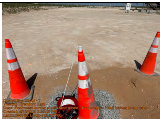
Northwest corner of pad facing east. Dry borehole 109.5 inches to top of casing.
