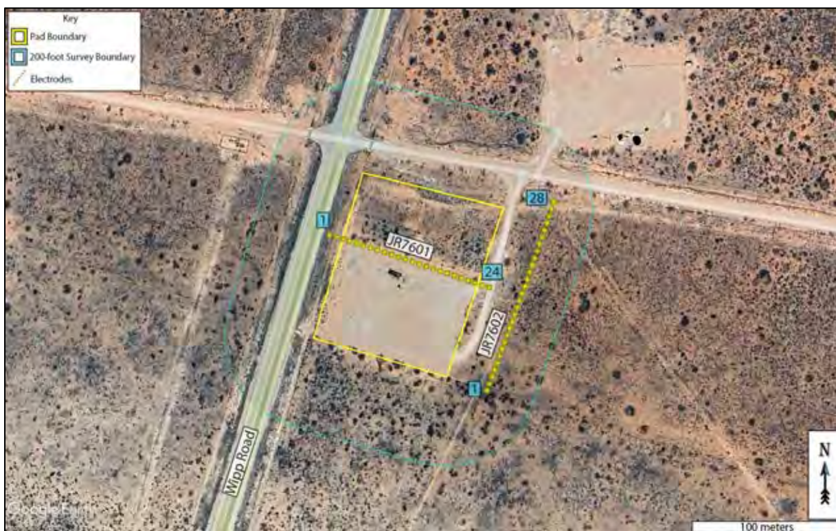
Figure 5: Geophysical survey overview. Two survey lines were conducted with 24 electrodes (JR7601) and 28 electrodes (JR7602), each at 5-meter spacing (yellow dots denoted with blue numbers). Background image credit: Google Earth. Image date: April 2, 2023. Image datum: WGS-84.
