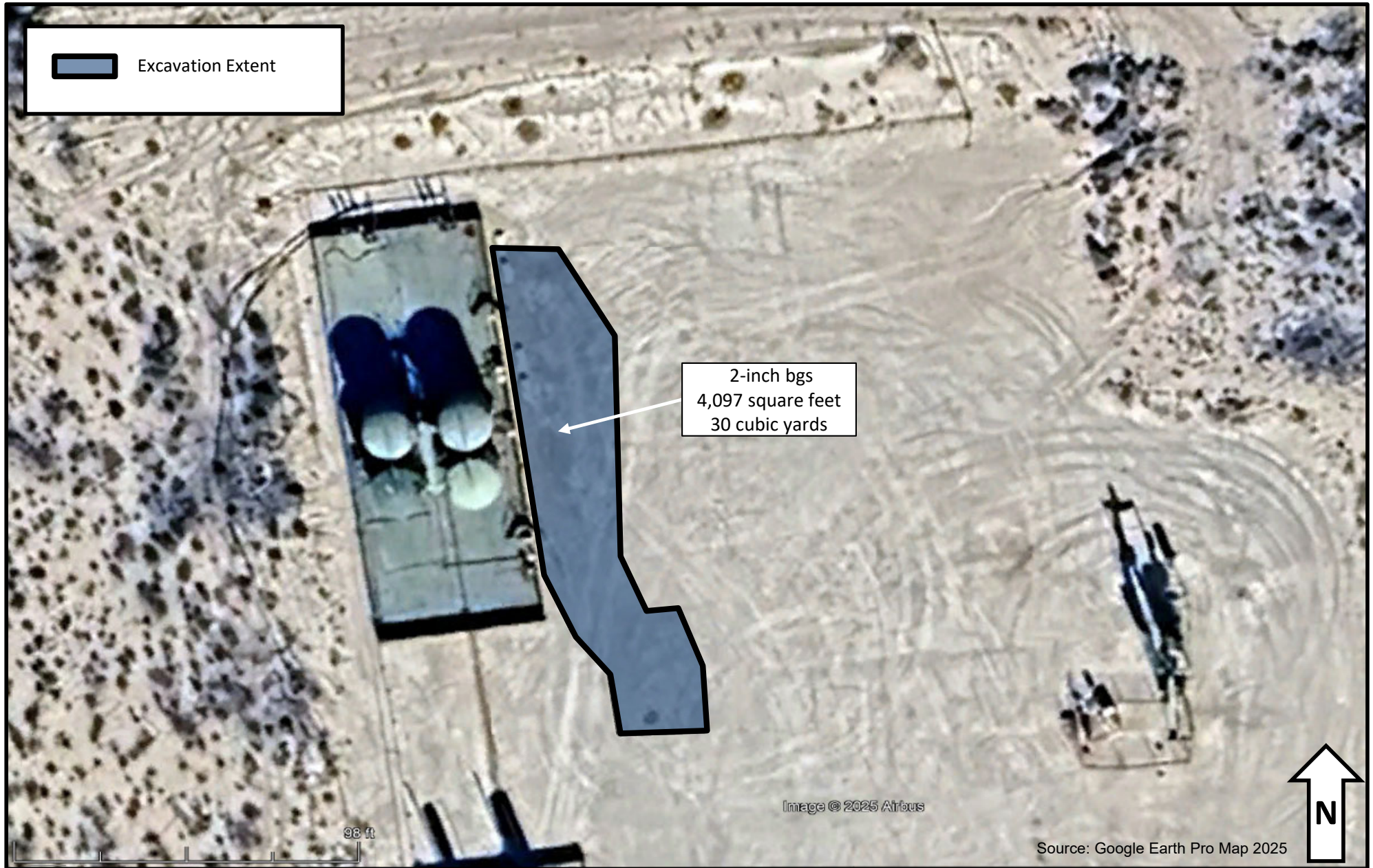
Figure 4 – Proposed Excavation Extent
