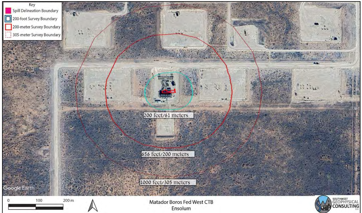
Figure 4: Surface karst survey overview. Background image credit: Google Earth. Image date: December 31, 2023. Datum: WGS-84.
