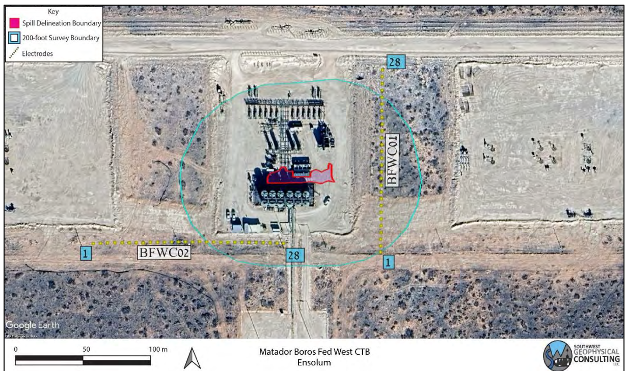
Figure 5: Geophysical survey overview. Two survey lines were conducted with 28 electrodes (yellow dots denoted with blue numbers). Background image credit: Google Earth. Image date: December 31, 2023. Datum: WGS-84.
