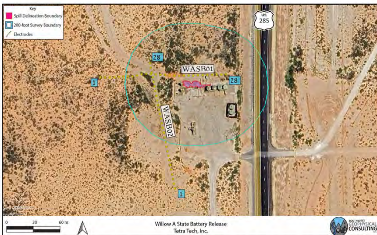
Figure 5: Geophysical survey overview. Two survey lines were conducted with 28 electrodes at 5-meter spacing (yellow dots denoted with blue numbers). Background image credit: Google Earth. Image date: July 13, 2024. Image datum: WGS-84.
