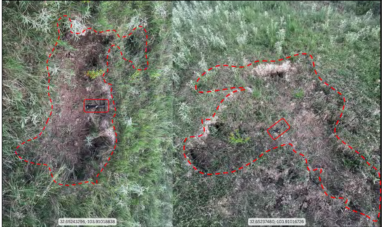
Figure 10. Photographs collected during the pedestrian karst survey on July 29, illustrating irregular soil collapse features formed by subsurface erosion processes. A hammer (highlighted by the red rectangle; length 15.28 in) is included for scale.
