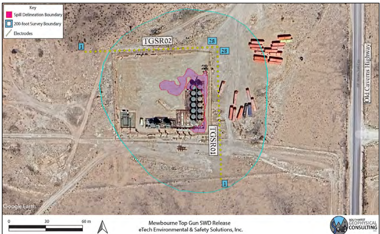
Figure 5: Geophysical survey overview. Two survey lines were conducted with 28 electrodes each at 5-meter spacing (yellow dots denoted with blue numbers). Background image credit: Google Earth. Image date: April 15, 2023. Image datum: WGS-84.
