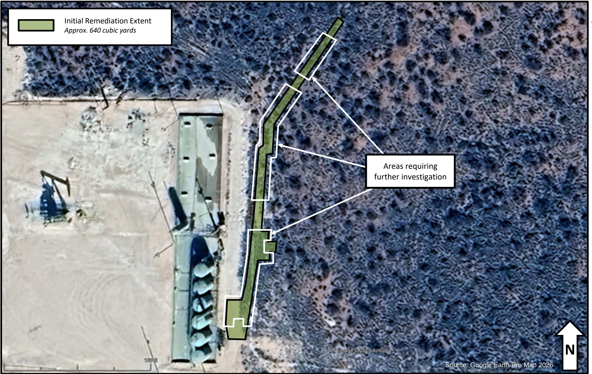
Figure 2 – Initial Remediation Extent
