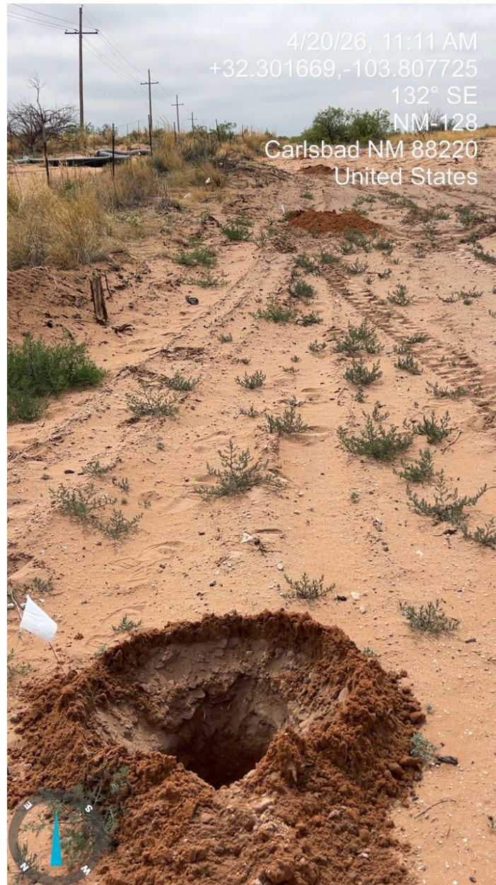
Photograph showing a completed boring of delineation sample locations, viewing southeast.
