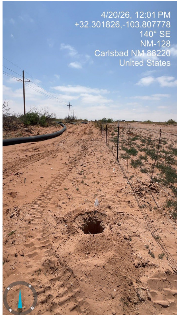
Photograph showing a completed boring of a delineation sample location, viewing southeast.
