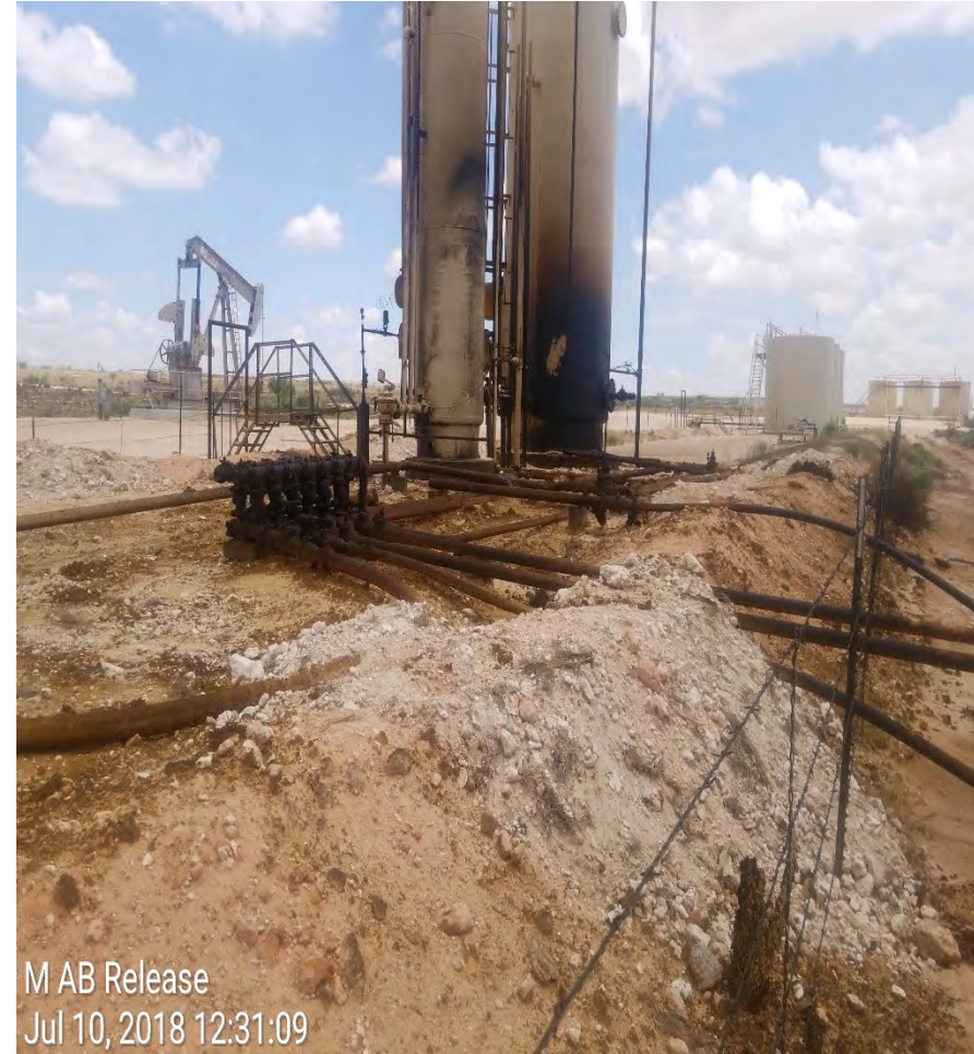
View Northeast– A portion of the spill flow path caused by the fluid release. Note the hydrocarbon staining (dark brown).
