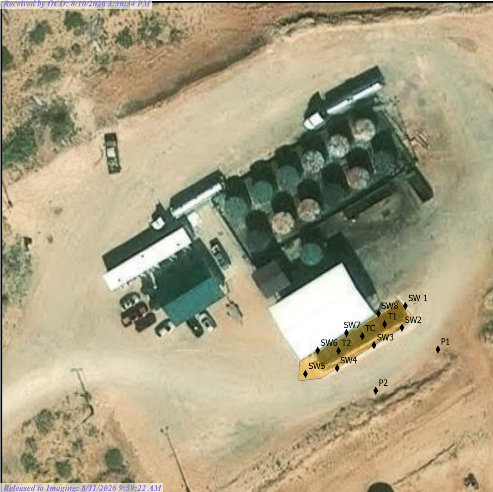
FIGURE 1 Excavation Area Sandpoint BGT removals
