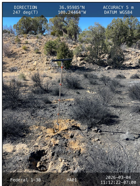
Photograph: 3 Description: Hand auger boring HA01, advanced within the release footprint and adjacent to a potential point of release.
