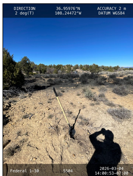
Photograph: 7 Date: 03/04/2026 Description: Surface sample SS04, taken outside the release footprint to laterally delineate the release extent. View: North
