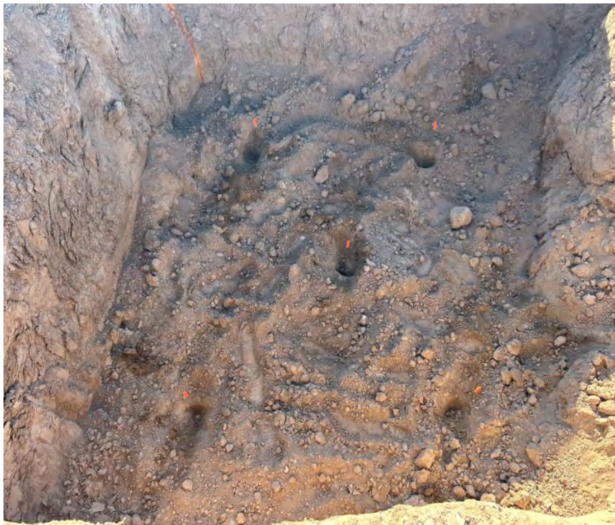
View of the base of the excavation with 5-point sample collection.
