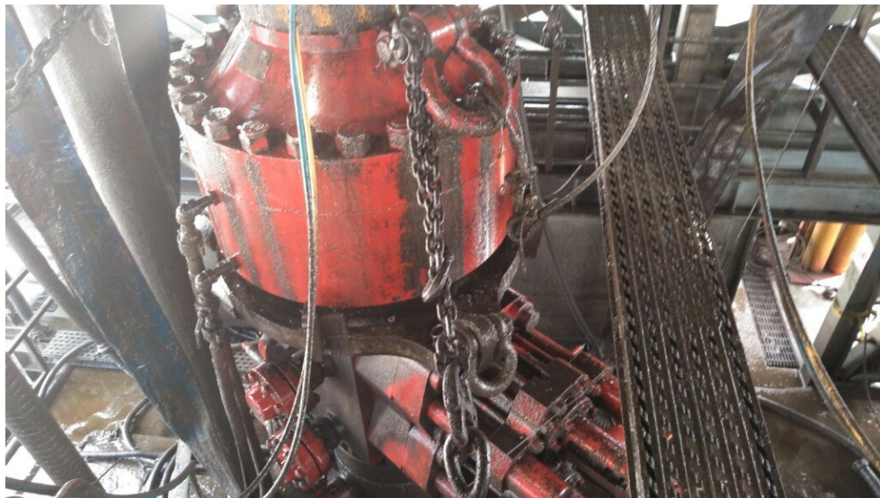
Figure 1: Winch System attached to BOP Stack
