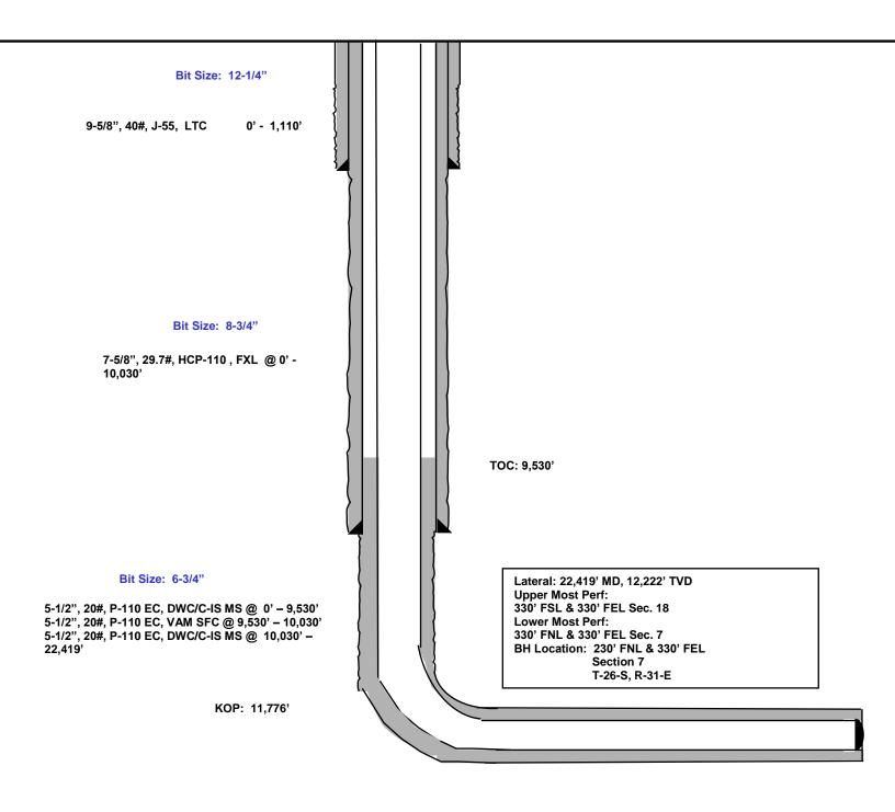
319' FSL 1,145' FEL Section 18 T-26-S, R-31-E Proposed Wellbore Design B KB: 3,220' GL: 3,195'
