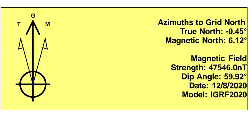
To convert a Magnetic Direction to a Grid Direction, Add 6.12°
