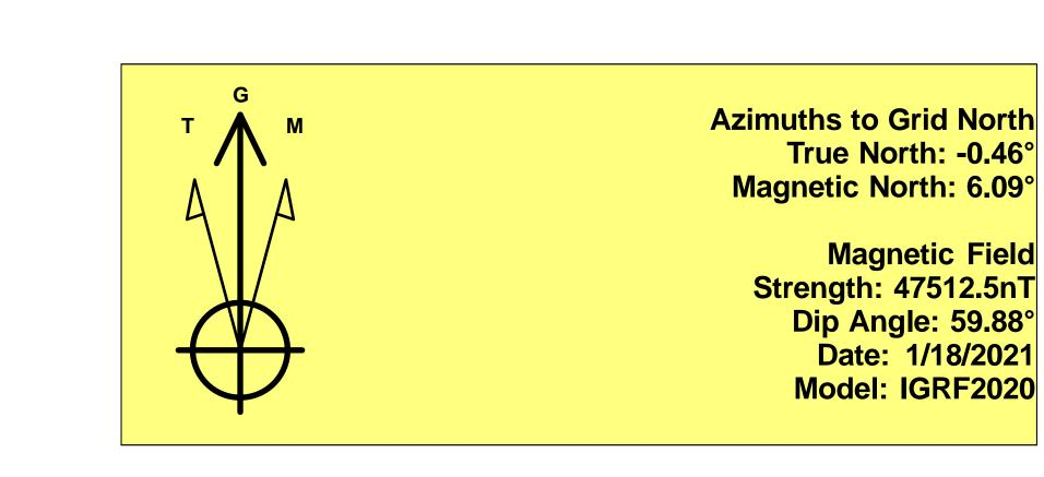
To convert a Magnetic Direction to a Grid Direction, Add 6.09° To convert a Magnetic Direction to a True Direction, Add 6.54° East To convert a True Direction to a Grid Direction, Subtract 0.46°
