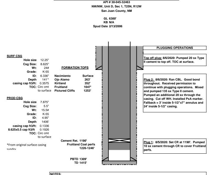
A-Plus Rig 9: MOLRU on 8/5/2020. SITP=0 psi. SICP=10 psi. SIBHP=0 psi. Set CR at 1190'. PT casing to 600 psi. Test failed. Hole appeared in BH during PT. Ran CBL. Good bond throughout. Received approval to continue operations. All plugs Type II cement mixed at 15.6 ppg, yield 1.18 cu. ft./sack. Regulatory representative on site: Clay Yazzie Attached are the PxA marker photo and the GPS coordinates Plugging and abandonment was completed on 8/6/2020 and the rig was released.
