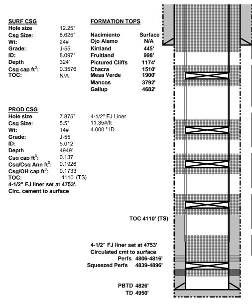
Plug 6: Perf 4 holes at 495'. Tie onto 5-1/2" casing. Mix and pump sufficient cement to bring cement to surface, inside and outside 4-1/2" liner, to cover tops of Kirtland, Ojo Alamo, surface casing shoe, and surface plug inside and outside.
