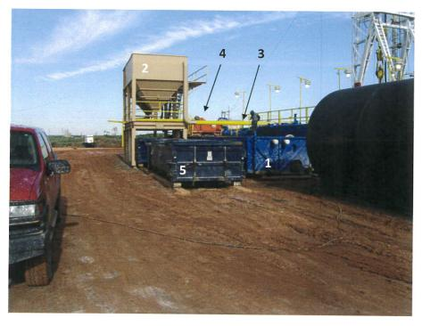
Closed Loop Drilling System: Mud tanks to right (1)
