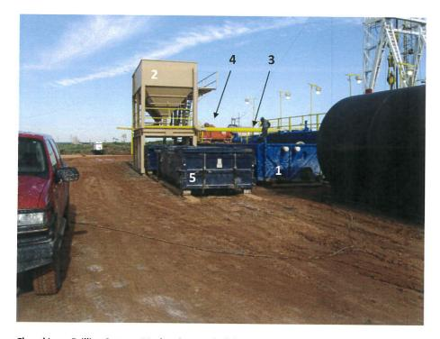
Closed Loop Drilling System: Mud tanks to right (1) Hopper in air to settle out solids (2) Water return pipe (3) Shaker between hopper and mud tanks (4)
