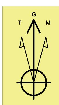
Azimuths to Grid North True North: -0.23° Magnetic North: 6.58°
