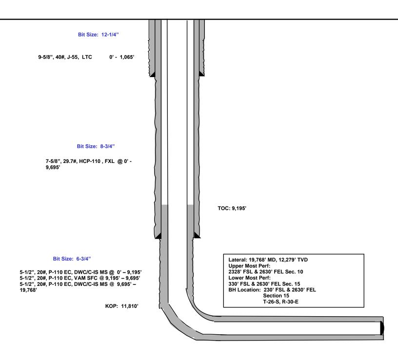
2539' FSL 2440' FWL Section 10 T-26-S, R-30-E Proposed Wellbore Design B KB: 3,155' GL: 3,130'
