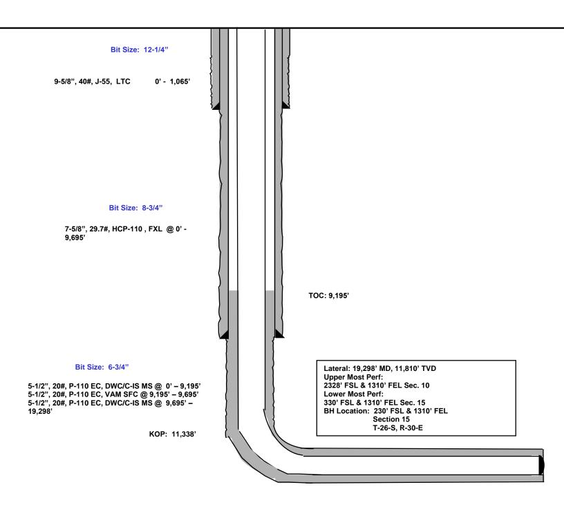
2579' FSL 1534' FEL Section 10 T-26-S, R-30-E Proposed Wellbore Design B KB: 3,176' GL: 3,151'
