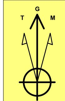
Azimuths to Grid North True North: -0.29° Magnetic North: 6.46°
