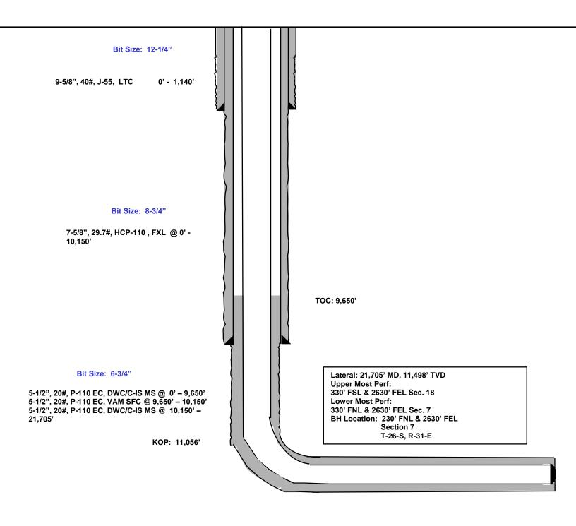
826' FSL 2396' FWL Section 18 T-26-S, R-31-E Proposed Wellbore Design B KB: 3,208' GL: 3,183'
