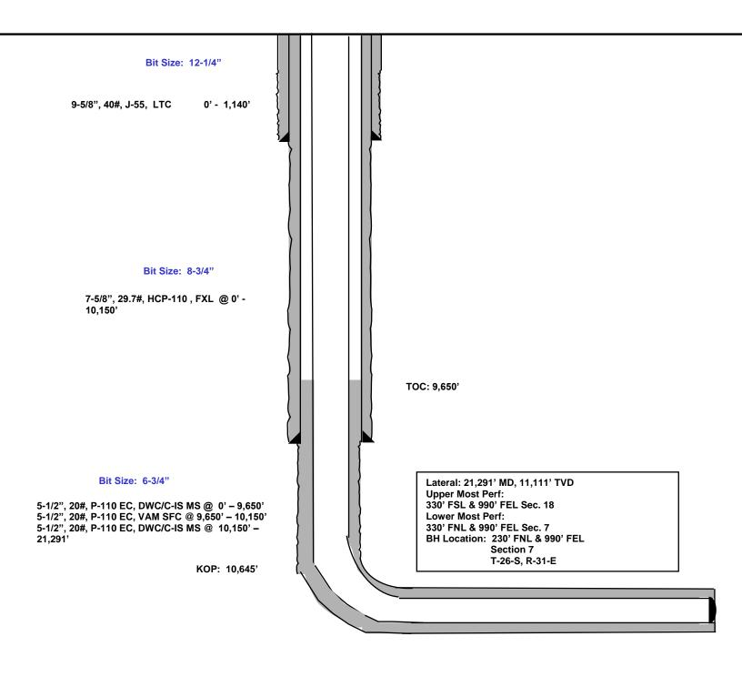
201' FSL 1421' FEL Section 18 T-26-S, R-31-E Proposed Wellbore Design B KB: 3,217' GL: 3,192'
