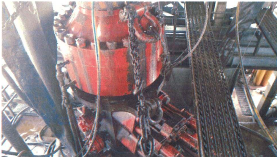
Figure 1: Winch System attached to BOP Stack
