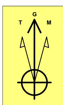
**Azimuths to Grid North** True North: -0.29° Magnetic North: 6.45°
