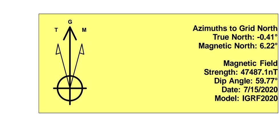
To convert a Magnetic Direction to a Grid Direction, Add 6.22° To convert a Magnetic Direction to a True Direction, Add 6.63° East To convert a True Direction to a Grid Direction, Subtract 0.41°
