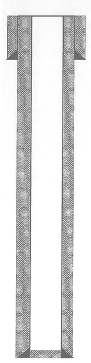
8-5/8", 24# J-55 Casing set @ 153' RKB Cemented w/ 164 sks Class B cement w/ 2% Calcium and ¼#/sk CF Circulated 8 bbl cement to surface
