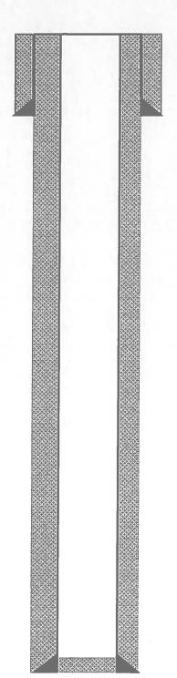
8-5/8", 24# J-55 Casing set @ 153' RKB Cemented w/ 164 sks Class B cement w/ 2% Calcium and ¼#/sk CF Circulated 8 bbl cement to surface
