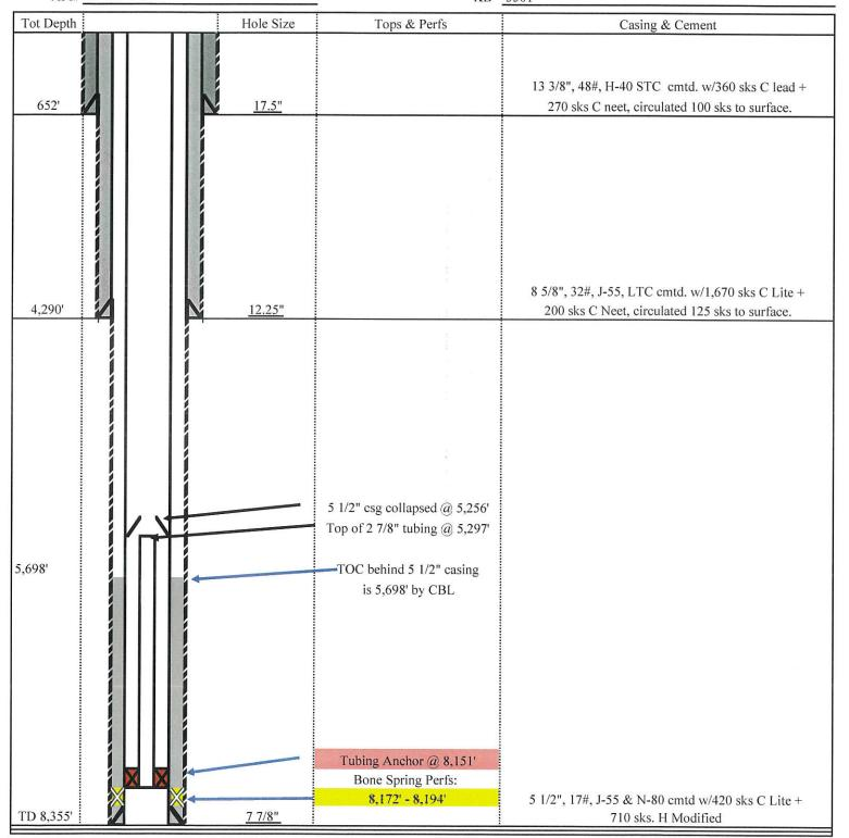
REMARKS: 5 1/2" casing collapsed @ 5,256'; unable to sweage out same. Cut off top of 2 7/8" tubing string is 5,297'.
