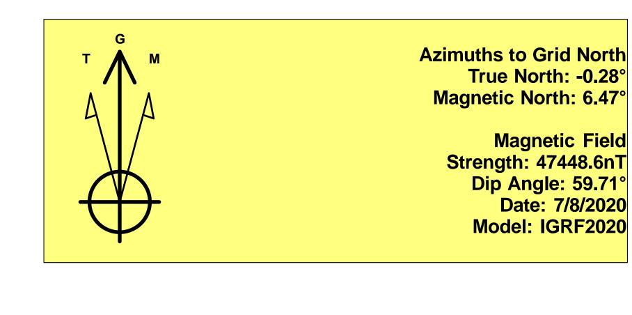
To convert a Magnetic Direction to a Grid Direction, Add 6.47° To convert a Magnetic Direction to a True Direction, Add 6.75° East To convert a True Direction to a Grid Direction, Subtract 0.28°
