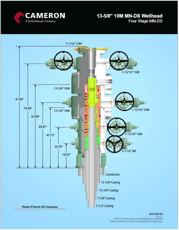
Wellhead shall be installed by Cameron representative. Cameron rep shall install the test plug for the initial BOP test.
