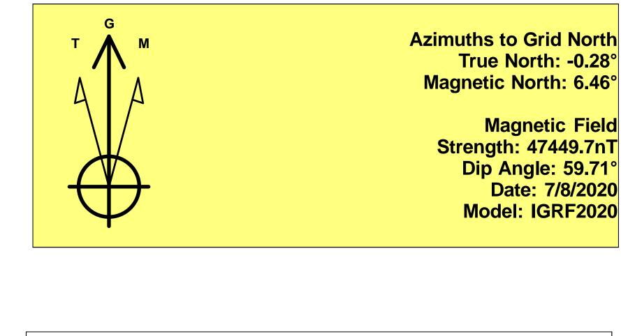
To convert a Magnetic Direction to a Grid Direction, Add 6.46° To convert a Magnetic Direction to a True Direction, Add 6.75° East To convert a True Direction to a Grid Direction, Subtract 0.28°
