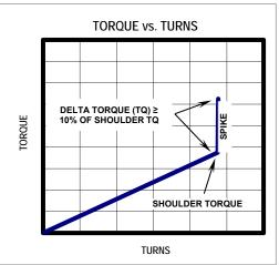
When using Torque vs. Turn monitoring equipment, GB recommends setting a reference torque value of 500 ft.-lbs. or 10% of the minimum makeup torque (whichever is lower) to normalize the resulting plots. Plot scales should be set so data spans at least 2/3 of the turns scale on each plot (15 turns will usually be sufficient at the start and can be reduced based on data from the first few joints). UNDER NO CIRCUMSTANCE SHOULD MAKEUP BE STARTED UNTIL THE MONITORING SYSTEM IS READY TO RECORD DATA.
