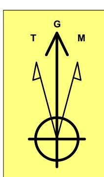
Azimuths to Grid North True North: -0.29° Magnetic North: 6.45°
