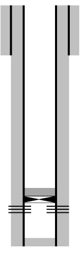
12-1/4" hole @ 714' 8-5/8"24# csg @ 708' w/ 400sx-TOC-Surf-Circ.
