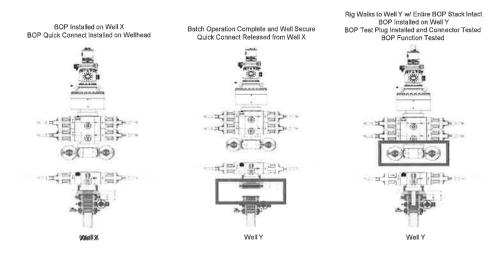
Note: Picture below highlights BOP components that will be tested during batch operations
