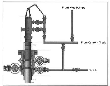
Wellhead diagram during offline cementing operations
