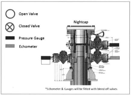
Wellhead diagram during skidding operations
