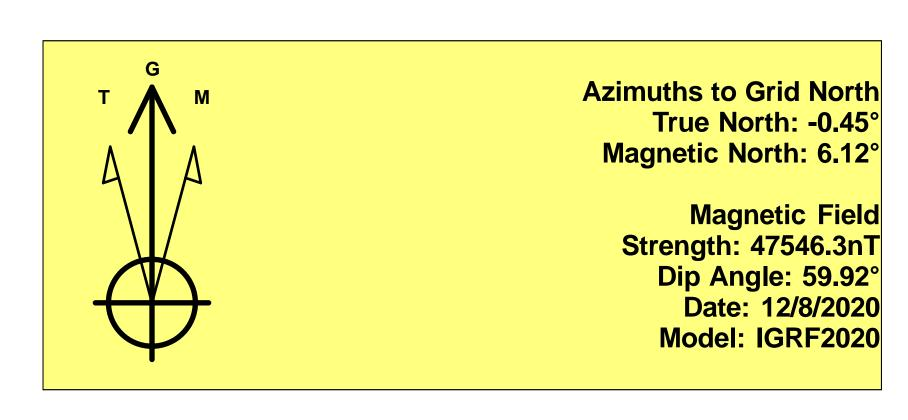
To convert a Magnetic Direction to a Grid Direction, Add 6.12° To convert a Magnetic Direction to a True Direction, Add 6.57° East To convert a True Direction to a Grid Direction, Subtract 0.45°
