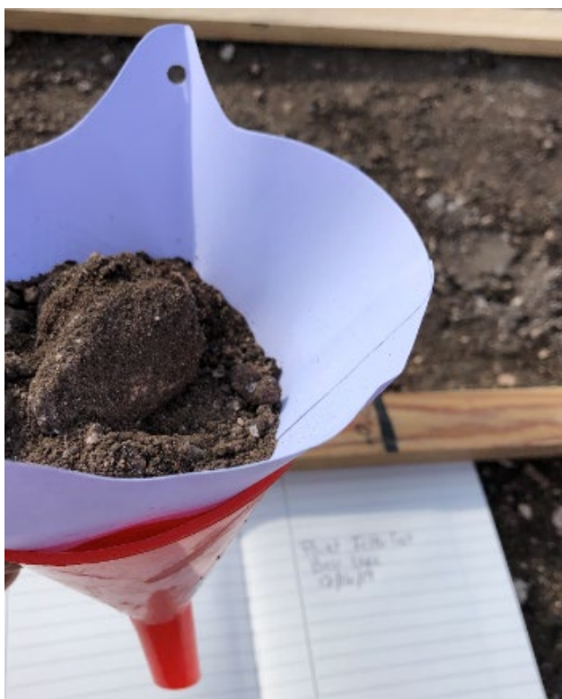
Figure 3 - Paint Filter Test (12-16-19)
